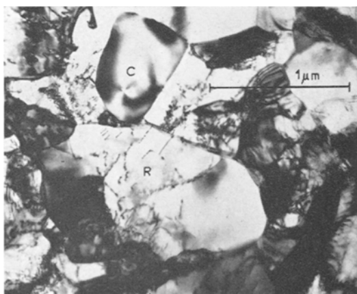
Figure 2 Electron micrograph of a recrystallised grain associated with a carbide particle ( \times 25,000 ).
